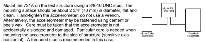
Depress POWER SWITCH of the P31 Power Unit/Amplifier to TEST position. BATTERY CONDITION INDICATOR should show a steady green light, release switch. Connect the cable to the input connector on the P31 and to the 731A seismic accelerometer. This cable should be free of kinks and cable connectors should be clean. Connect one end of a coaxial cable to the output BNC connector on the rear panel of the P31 and connect the other end of the cable to the readout or recording instrument.
