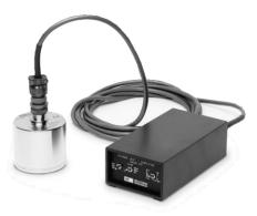
This system is particularly suited for the measurement of low level vibrations in bridge, building, tower and dam motion studies, optical and photographic stability monitoring, electron microscope and microtome monitoring, as well as vibration-isolation table monitoring.
