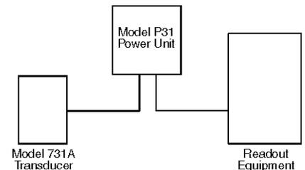
Depress POWER SWITCH of the P31 Power Unit/Amplifier to TEST position. BATTERY CONDITION INDICATOR should show a steady green light, release switch. Connect the cable to the input connector on the P31 and to the 731A seismic accelerometer. This cable should be free of kinks and cable connectors should be clean. Connect one end of a coaxial cable to the output BNC connector on the rear panel of the P31 and connect the other end of the cable to the readout or recording instrument.
