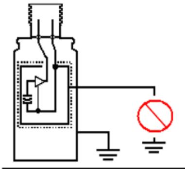
Figure 3: Electrical characteristics of IEPE sensors
