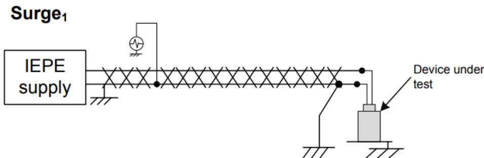
Then surge energy was applied to the accelerometer signal lines A and B. For this test, visible damage occurred to the printed circuit board assembly. This failure mode was not consistent with the failures seen in wind turbine applications.
