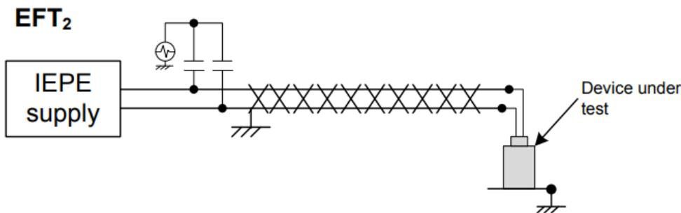
For the surge immunity test, energy was coupled to the sensor cable shield, both grounded and ungrounded. Under this configuration, no damage was sustained to the accelerometer.
