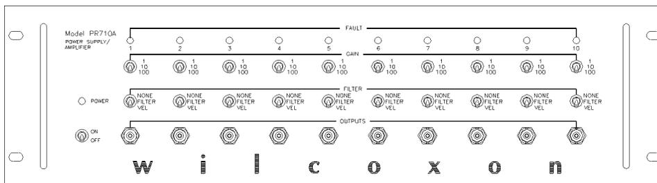
The PR710 is specifically designed to furnish the constant DC current necessary to operate the internal amplifier of piezoelectric transducers (accelerometers and velocity sensors), which require a constant current power supply.
