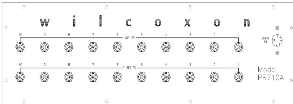
**Caution:** The PR710B input connectors are twin-axial BNC connectors. Attempting to force a standard co-axial BNC into the twin axial BNC will damage the input connector.
