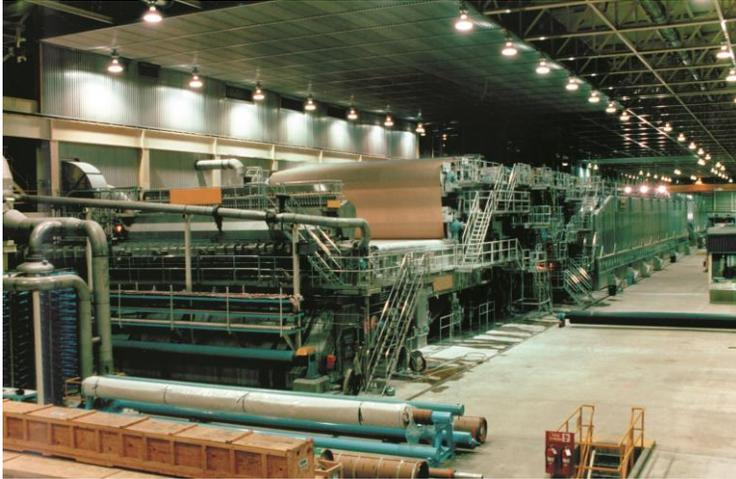
Successful vibration monitoring of paper machines depends on quality sensors, field proven for reliability. Accelerometers used in paper mill applications must survive harsh thermal, electrical and chemical environments while performing demanding bearing measurements. Wilcoxon piezoceramic accelerometers are the sensor of choice for accurately measuring the broad range of frequencies and low amplitudes occurring in slow speed roller bearing installations.
