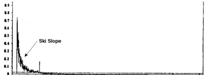
Figure 6b: Overload operation
