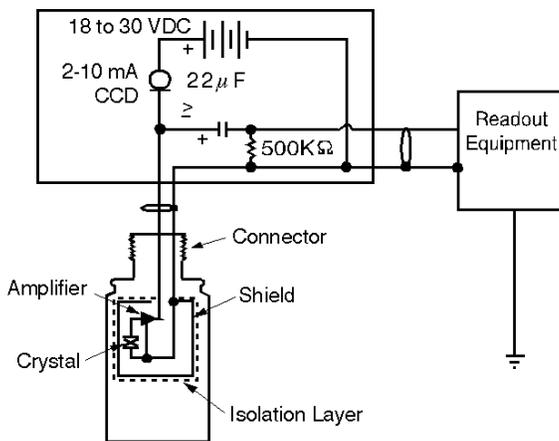
Figure 3: Schematic of a sensor power supply
