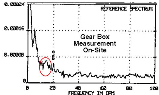
Figure 7: Ski-slope noise caused by analog integration
