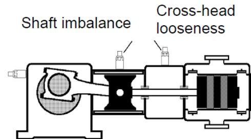
Figure 3: Mounting locations for sensors
