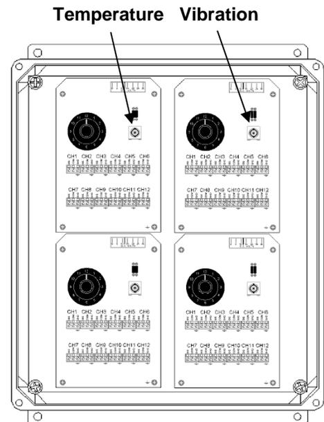
The shield must be wired to at least one shield connection point, but it is not necessary to connect it to both channel's shield connection. The temperature and the acceleration signals share the common connection. Illustrated here is a VL48EX switch box that will allow access to both signals for vibration and temperature sensors such as the 786T.
