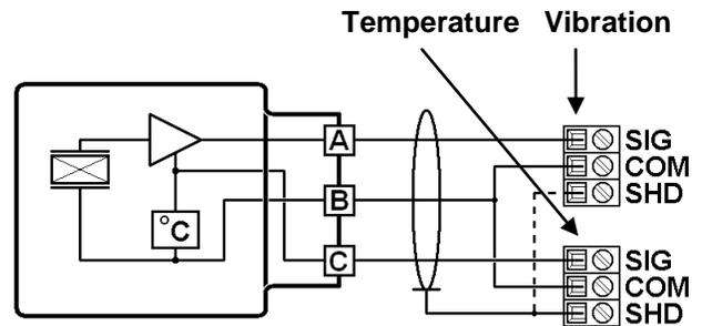
When wiring the shield, it only needs one termination point.
