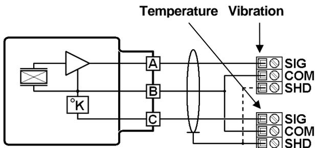
The shield (SHD) connection to an on-line system must connect to the system reference ground.
