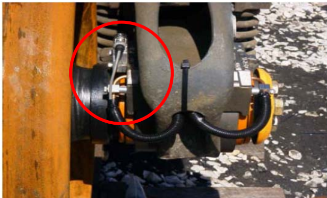
Wilcoxon Research model 787A mounted on the bearing adaptor of a caboose
