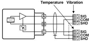
The shield (SHD) connection to an on-line system must connect to the system reference ground.
