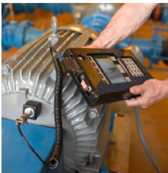
Portable data collection with route-based tools utilizes a single accelerometer and requires extensive training
