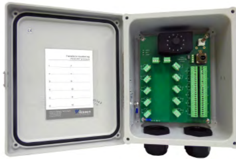
Single channel and triaxial switchboxes
