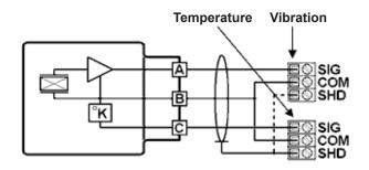
The accelerometer and temperature sensors are each wired to their own channel. The sensors share the same common connection, so it must be split and wired to each channel's common connection. When wiring the shield, it only needs one termination point. The voltages developed at the terminals of the sensor are shown in the table in the appendix of this guide. All readings are in °K.
