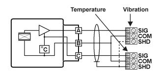
wilcoxon.com buy.wilcoxon.com The 786T, when permanently installed for dual vibration and temperature measurements, should be wired to two channels of a vibration switchbox. The three-pin connections of the 786T are:
