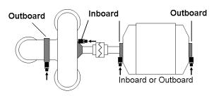
Figure 6: Top view of a motor-pump set with recommended mounting locations
