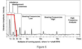
Wilcoxon offers special frequency banded 4-20 mA transducers. The PC420VP-10-B3041 uses high-pass and lowpass filters before the detection circuitry to focus the output detection to the range between 3 and 40 Hz (180 and 2400 CPM) to process and compute the vibration level output to the 4-20 mA process loop. This focus of analysis enables users to trend only the low frequencies of vibration associated with balance or alignment problems on most heavy machines.
