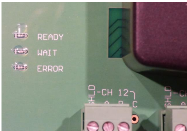
Figure 7: Upper left side of the VibraLINK® board showing the location of the status LEDs
