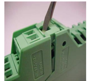
Figure 6 – Releasing the latch of the iT401 case
