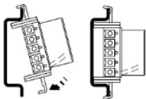
The completed connector assembly on the rail.
