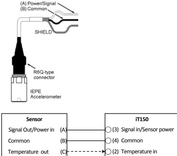
Figure 6 - Sensor connections
