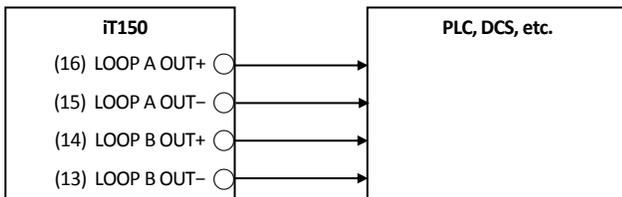
Figure 8 - 4-20 mA current loop connections
