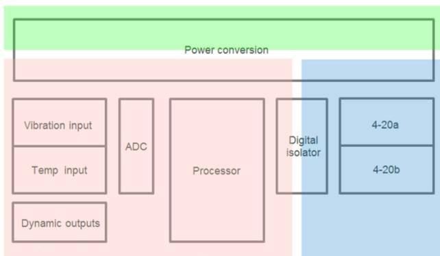
Figure 4 - Isolation diagram
