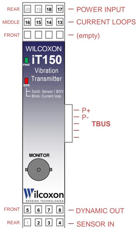
Figure 5 - IO port and terminal block locations
