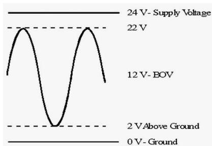
Figure 11 - Maximum input signal swing with 12V BOV
