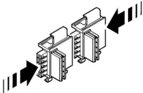
Attach the connectors to the DIN rail by hooking the latch of the connectors over the top of the rail and then snapping the bottom of the connectors onto the rail.
