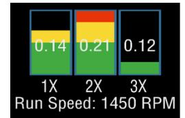
The display shows the vibration level in frequency ranges based on multiples, also known as orders, (1X, 2X and 3X) of the specified machine run speed shown beneath the bars.
