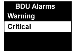
Both threshold values can be set independently using up and down arrows. The levels are typical for medium sized machine bearings operating at run speeds from 1000 to 3000 RPM. Larger bearings or higher run speeds may need increased BDU threshold values to identify worn or bad bearings.
