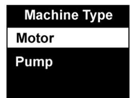
Selecting the machine type and size allows the ISO alarm levels to be set accordingly, as does specifying the type of mounting (rigid or flexible).
