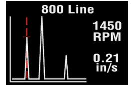
The heights of the peaks indicate RMS vibration level (mm/s or inch/s) at each frequency point in the spectrum.
