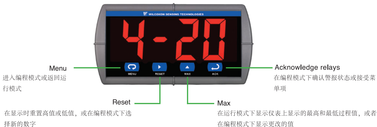
NEMA 4X / IP65 front panel
