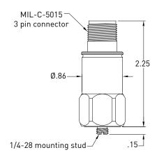
Notes: <sup>1</sup> Frequency response limits and spectral noise values are typical. Accessories supplied: SF6 mounting stud (metric mounting available); calibration data (level 2)
