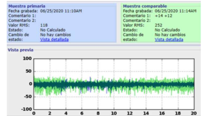
Pre-lubrication, normal bearing
