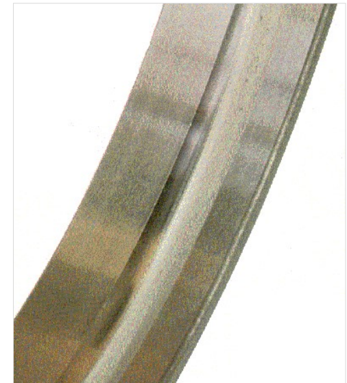
Wide ball path on inner raceway
