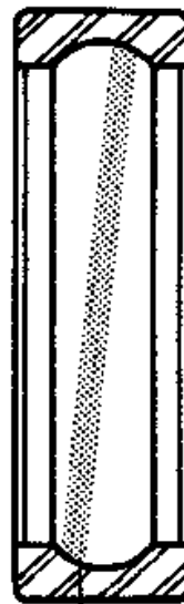
Non-parallel ball path on outer raceway
