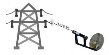
For electrical inspection of power lines, the range extender parabolic dish lets the operator detect airborne ultrasound up to 300' away.
