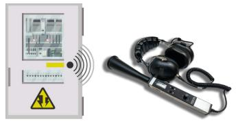
To hear airborne ultrasound created by electrical arcing and corona discharge, the receiver is used with acoustic concentrators that allow the operator to remain at a safe distance from the electrical cabinet, up to 150' away.
