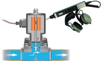
To hear structure-borne ultrasound created by leaky valves, the receiver is used with solid probes in direct contact with the machine.
