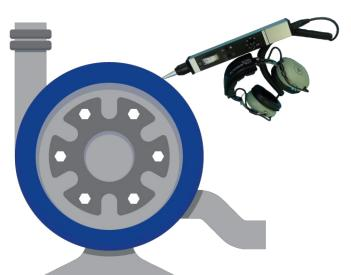
To hear structure-borne ultrasound created by bearings, gears, pumps, valves, and cylinders, the receiver is used with solid probes, which make direct contact with the machine being monitored.
