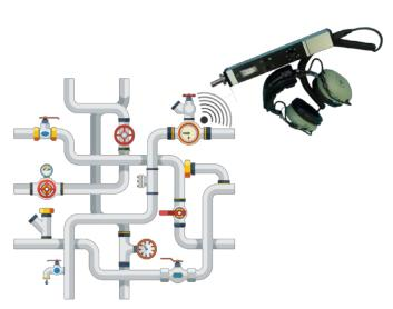
To hear airborne ultrasound created by turbulent flows, the receiver scans the exterior of the asset for leaks. Acoustic probes and concentrators allow the operator to remain at a safe distance from the asset being monitored, up to 150' away.
